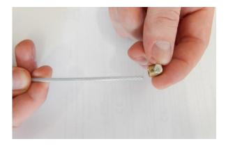
1. Put sleeves on the cable guides Img. 1. Place a screw in the sleeve, and best with fingers secure it until first resistance, then use flat wrench Img. 2 - and make 2 full turns. Making more turns wil damage the screw head.
